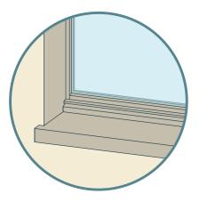
Whilst many imitation sash windows are installed on the outer frame, our range are installed recessed behind the frame to give the perceived 'depth' of sash.
